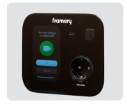
**UI Panel** From the UI Panel, you can adjust the pod's lighting and ventilation according to your personal preferences. Choose from Work Mode or Video Mode lighting presets, or control the brightness of both lights individually. The integrated 4G module enables to see the pod's availability, and make reservations directly with the *Bookable Pods* functionality on the touchscreen. Charge your devices via power outlets (1 power socket, USB C socket, optional LAN) located on the UI Panel.
